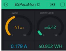
Fig. 5. Smart electricity monitoring for filament lamp
