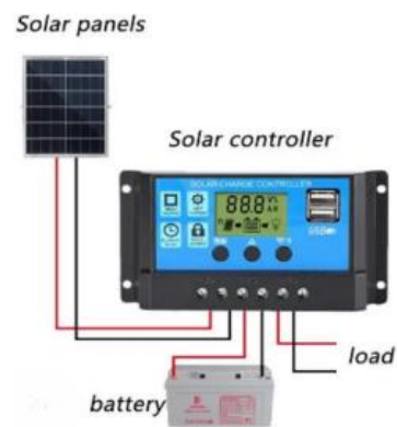
Fig. 7. Solar panel and PWM solar charge controller
